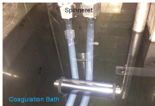
Figure 2. Photos of the fiber formation by encountering nonsolvent during the coagulation bath. [Color figure can be viewed in the online issue, which is available at wileyonlinelibrary.com.]
